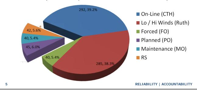
Rates are different than factors. Factors deal with a percent of the whole pie and Rates deal with a portion of the pie. Usually, the portion that the turbine is expected to run. It is expected that for Forced Outage Rate (FOR), On-Line, RUTH and Forced Outage the turbine should be running. It is not expected to run during Reserve Shutdown, Maintenance and Planned outages. So in the case of a Rate the denominator is smaller than a Factor.
