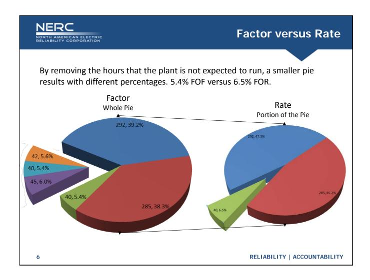
Notice the green slice percent changes from a factor of 5.4% to 6.5% for the rate. This is because the denominator is smaller in the rate calculation. The rate calculation indicates the percent that the turbine was in Forced Outage when it should have been running. The factor calculation indicates the percent of Forced Outage whether the turbine was running or not.
